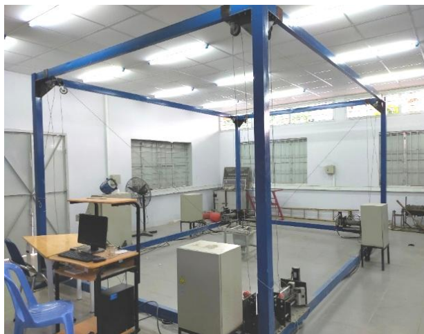
Figure 11. Cable robotic system in experiments.
