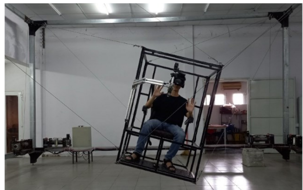
Fig.2. Cable Suspended Parallel Robot employs 8 cables to manipulate the object.
